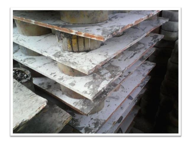
PolyBoard is now replacing standard plywood sheets as stackers for Rubber-mould pavers. Though expensive compared to commercial plywood, PolyBoard has a longer life giving more cycles. ( Paver manufacturers had to change pylwood sheets every 4 weeks, PolyBoard has now lasted them over 6months.)
